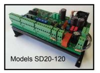
The EVACTRON SD series amplifier units are a new range of Building Occupant Warning System (BOWS) which provide Automatic and Manual control of Alert and Evacuation tones. The SD series units are available in a variety of sizes- 20, 40, 60,120 and 250 watt.
